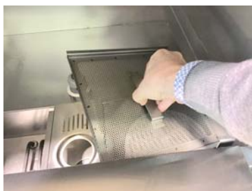
Remove the tank filters on the right
