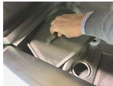
Remove the tank filters on the left
