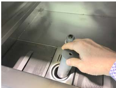
Remove the overflow pipe
