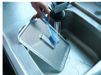
Clean the filter tank top
