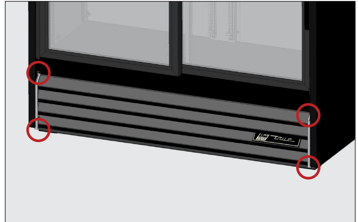
Fig. 2. Slide door louver grill screw location.
