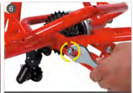
6. Tighten the nuts.
