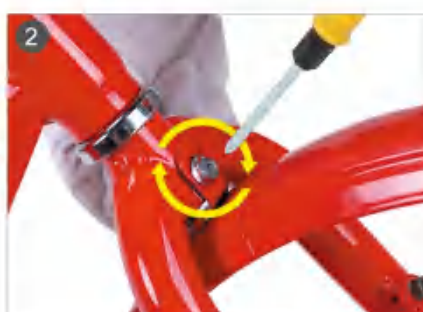
2. Tighten the screw.
