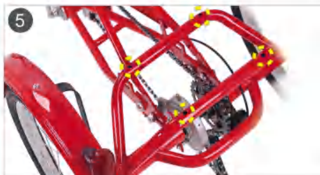
5. Four holes for fixing basket.
