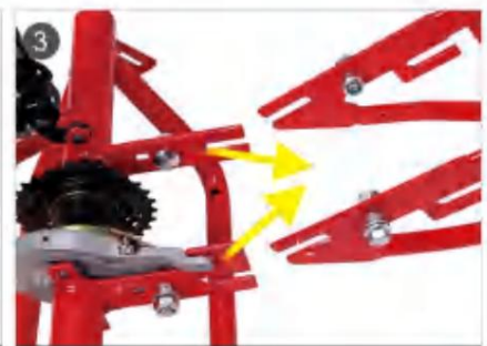
3. Assemble rear axle and frame.
