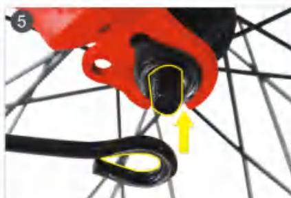
5. Assemble the fender holder.
