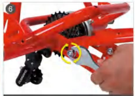
6. Tighten the nuts.
