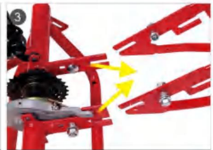
3. Assemble rear axle and frame.
