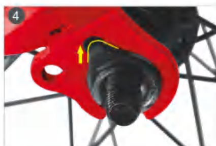
4. Assemble the washer.
