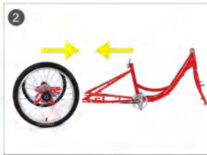
2. Connect the rear axle and frame, as shown.
