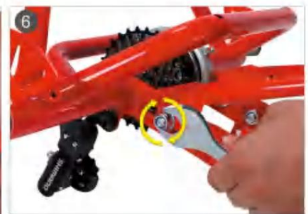
6. Tighten the nuts.
