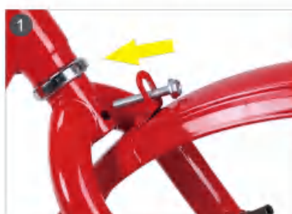
1. Assemble the front fender.
