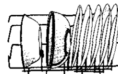
Flip away one section of plate tines to hold both bowls and plates.
