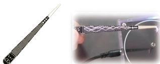
Lead pin: Hold the end of the lead pin and touch the lightning
