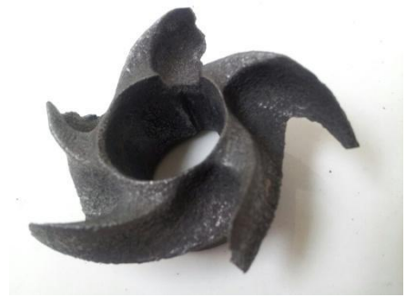
Impeller damaged from high acid solution
