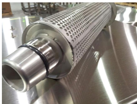
Pump filter and drain plug, note O-ring seal
