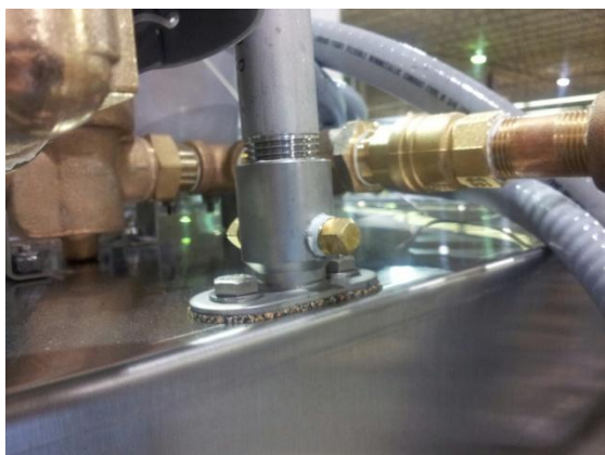
Mixing chamber with two 1/8" pipe threaded port
