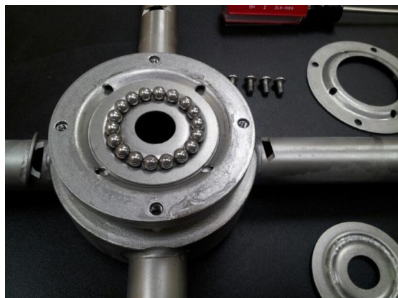
Top race removed, ball bearings for replacement
