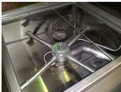
Wash arm w/bearing installed on base
