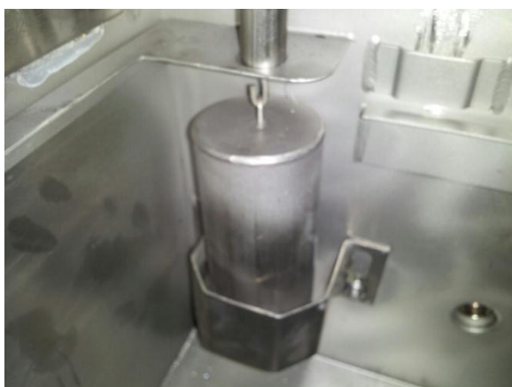
Wash tank float and tank overflow
