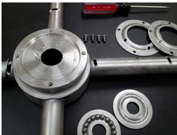
Races are interchangeable, capture shells are also
