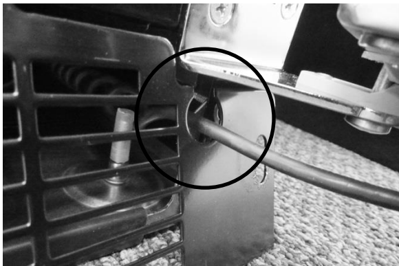
CORRECT Wire Position- Inside Grommet.
