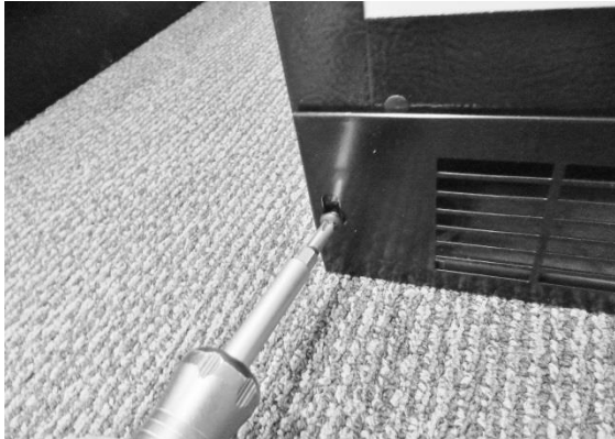
Remove each Phillip screws on both ends of the toe grill.
