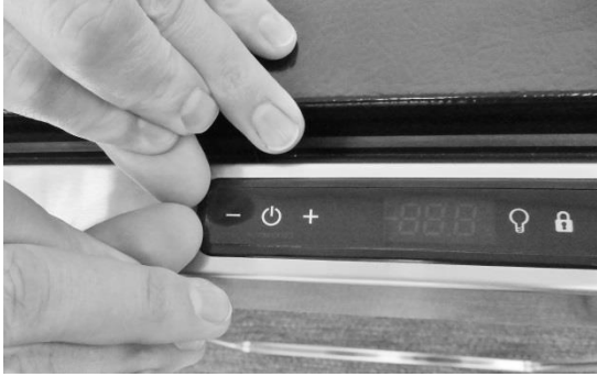
Place finger nails under left hand lip of user interface display.
