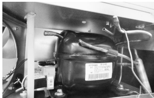
Cut the suction tube extension to connect the compressor to the suction line.
