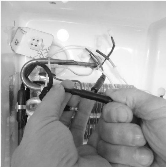
To replace defrost heater, unplug the connections.
