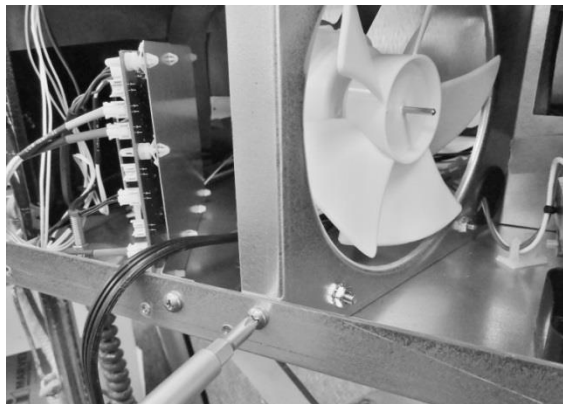
Remove bolt and nut.
