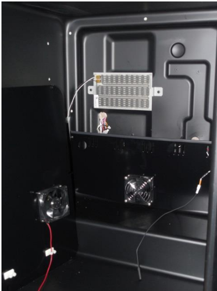
Upper Compartment Heater: Used to control and maintain the temperature of the upper zone.
