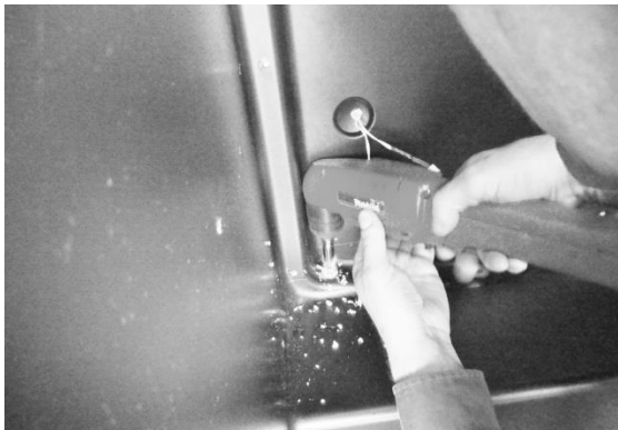
Drill a ½" hole downward into machine compartment. See recommendations in step 9 above.
