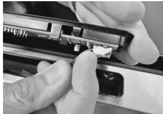
Release locking tab on display connector.
