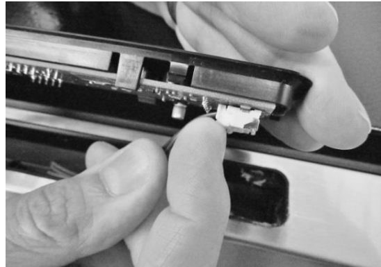
Release locking tab on display connector.
