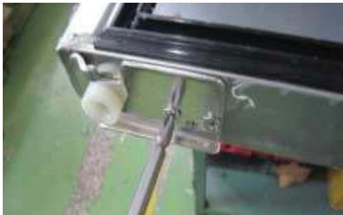
E. Disassemble stopper plate which located on bottom hinge (right), then assemble bottom hinge (right) on position of top hinge (left).
