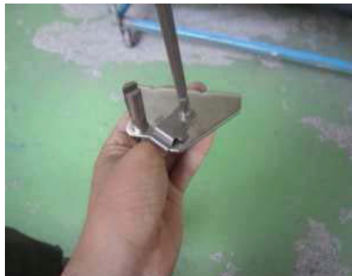
D. Screw stopper plate on top hinge (right).
