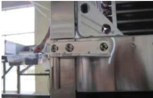
E. Disassemble stopper plate which located on bottom hinge (right), then assemble bottom hinge (right) on position of top hinge (left).
