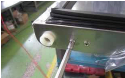
F. Disassemble stopper plate, then tight screws.
