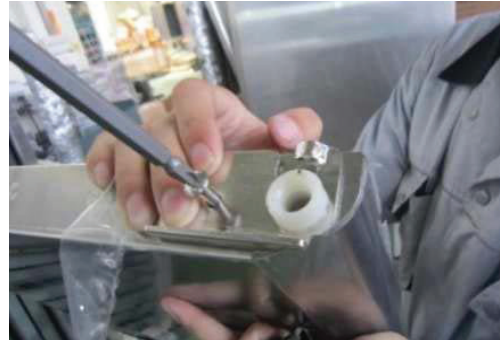
G. Assemble stopper plate in original positions.
