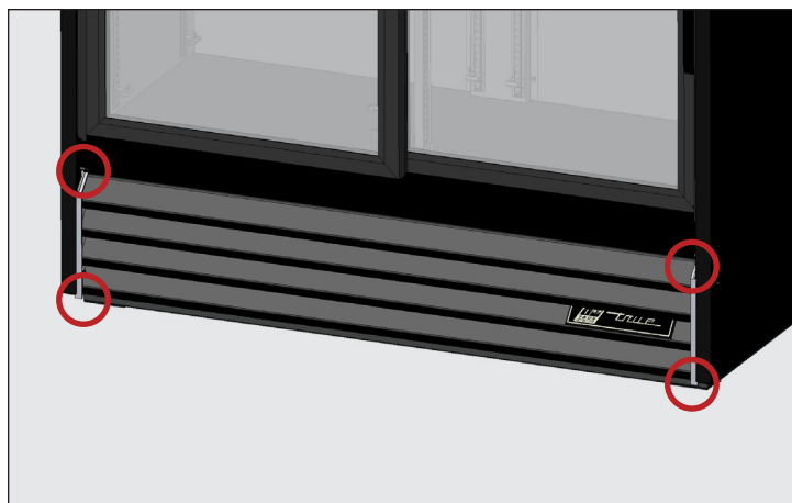
Fig. 2. Slide door louver grill screw location.
