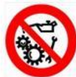
Prohibition to clean and lubricate moving parts
