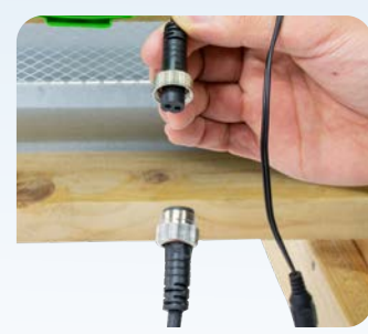
Connecting the Solar Panel
