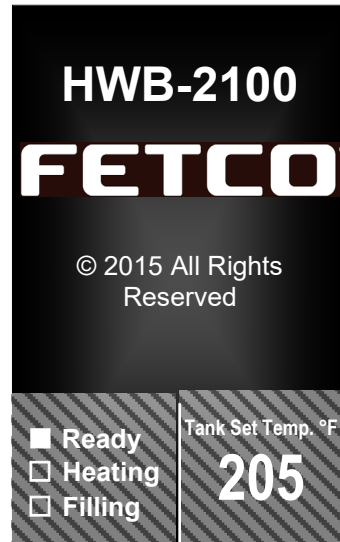
Hold finger on lower touch screen to access OPERATOR ACCESS SCREENS and programming menu screens
