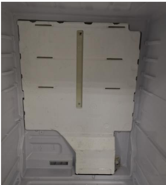
Refrigeration room air duct
