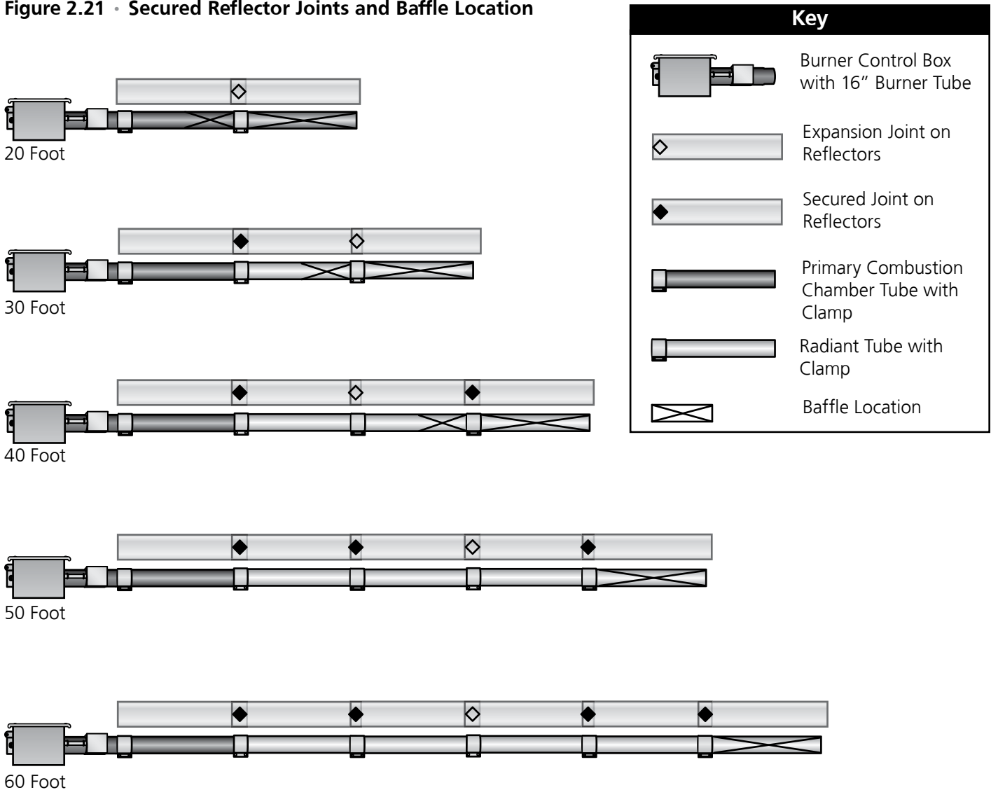
Figure 2.21 • Secured Reflector Joints and Baffle Location
