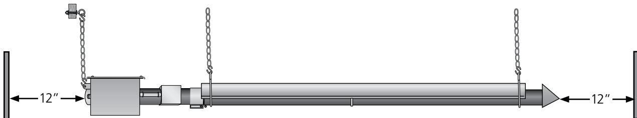
Figure 2.26 · Minimum End Clearance for Unvented Heater
