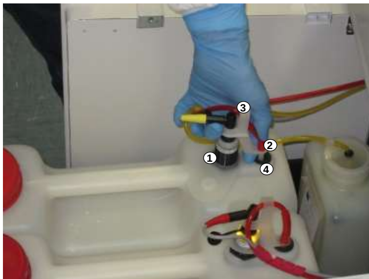
Figure 5-21: Removal of sensor and liquid tubing connectors
