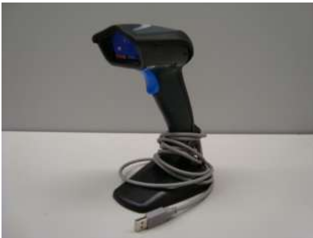
Figure 4-12: Handheld barcode reader (PN A0179 and PN A0256) with integrated support
