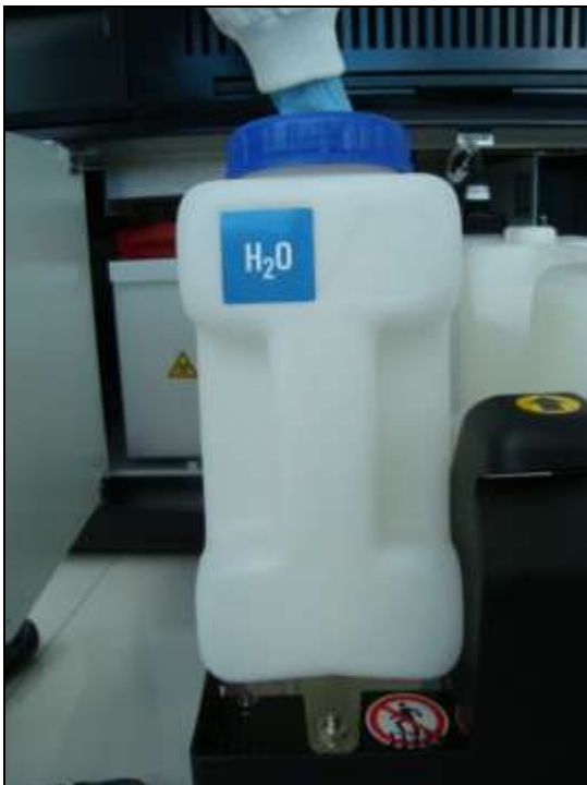
Figure 5-12: Raise water tank
