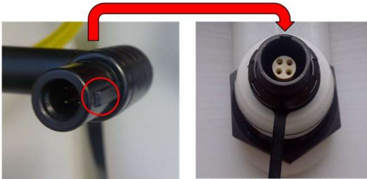
Figure 5-27: Sensor connector alignment
