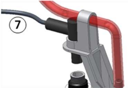
Figure 5-26: Sensor cable orientation
