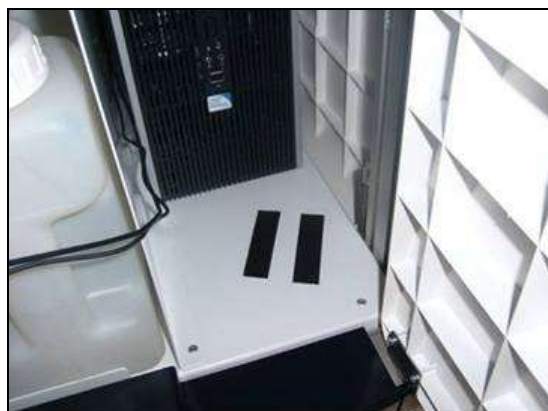
Figure 4-10: Velcro labels for barcode reader support (PN A0096)
