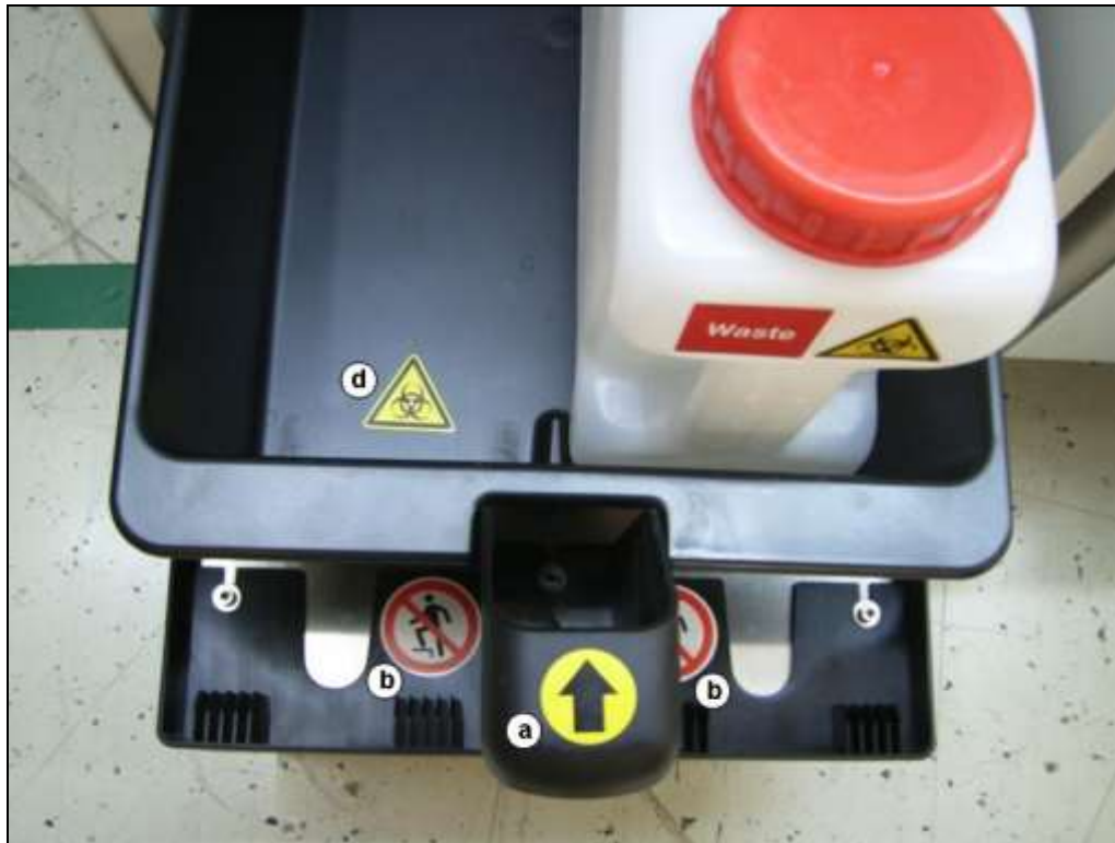
Figure 1-23: “Close”, “don’t step” and “bio-hazard” label positioning
