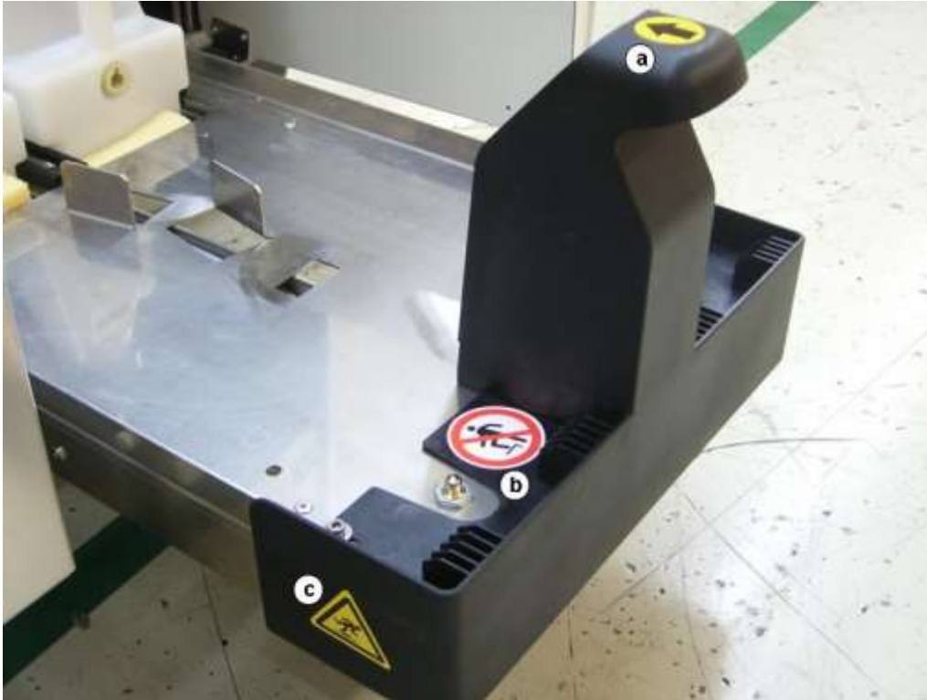
Figure 1-24: “Close”, “don’t step” and “stumble hazard” label positioning
