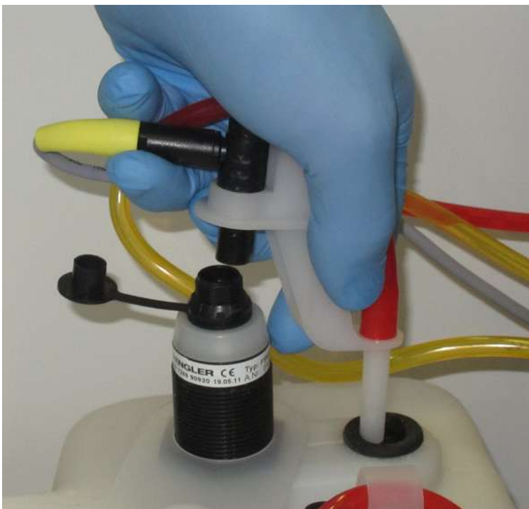
Figure 5-18: When disconnecting the sensor, the tubing is also pulled out of the membrane
