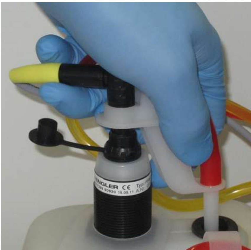
Figure 5-19: When pushing the tubing into the membrane, the sensor is also connected
