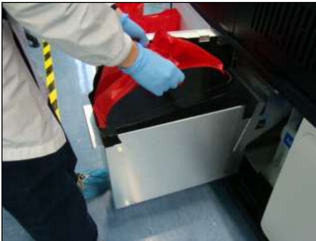
Figure 5-32: Waste bin and bag removal
