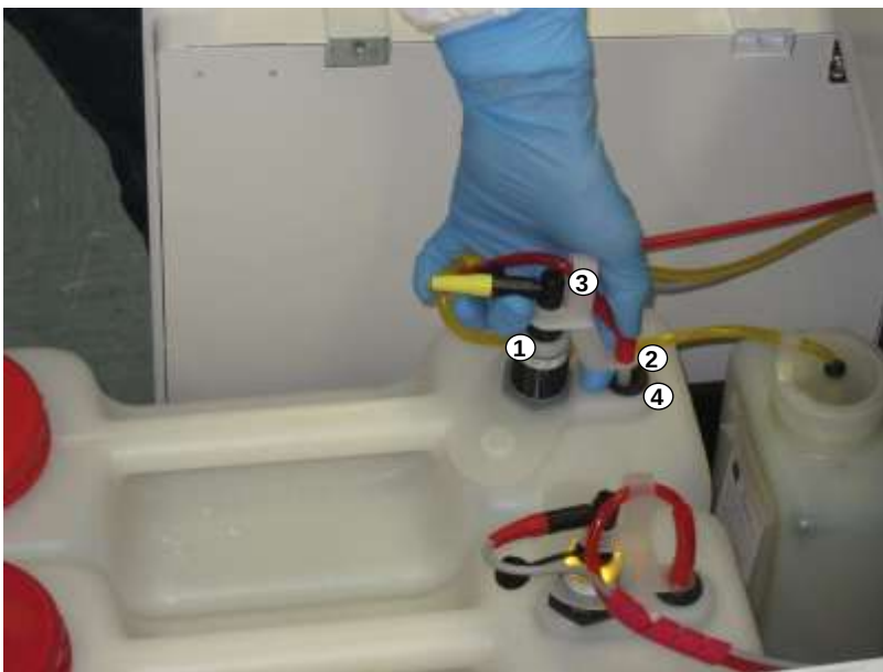
Figure 5-28: Insertion of sensor and liquid tubing connectors
