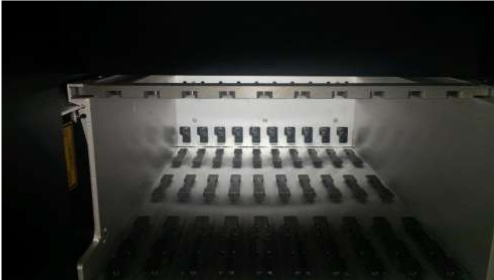
Figure 4-16: Sample bay not equipped with top cover
