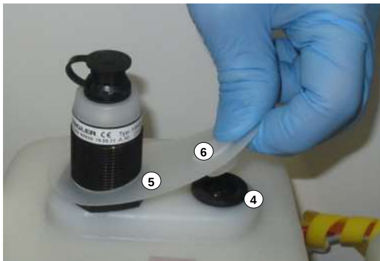
Figure 5-23: Rotation of the rubber strip and closure of the membrane with the cap
