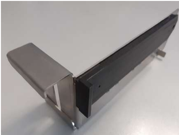
Figure 4-24 Ancillary rack with increased front wall and plastic block
