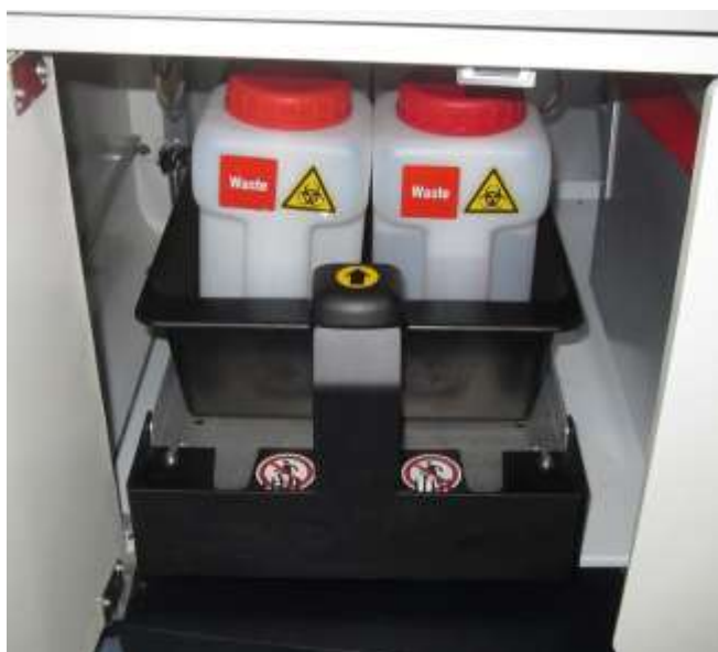
Figure 1-11: Liquid Waste tank and basin labels
