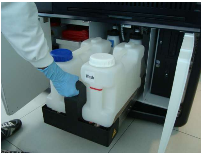
Figure 5-14: Right drawer insertion
