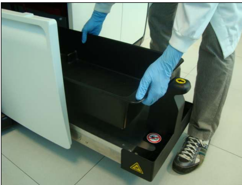
Figure 5-31: Waste basin removal
