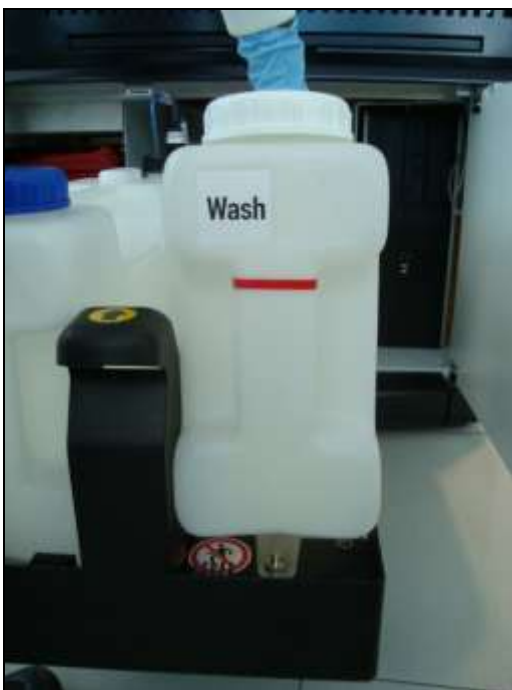
Figure 5-15: Raise wash buffer tank
