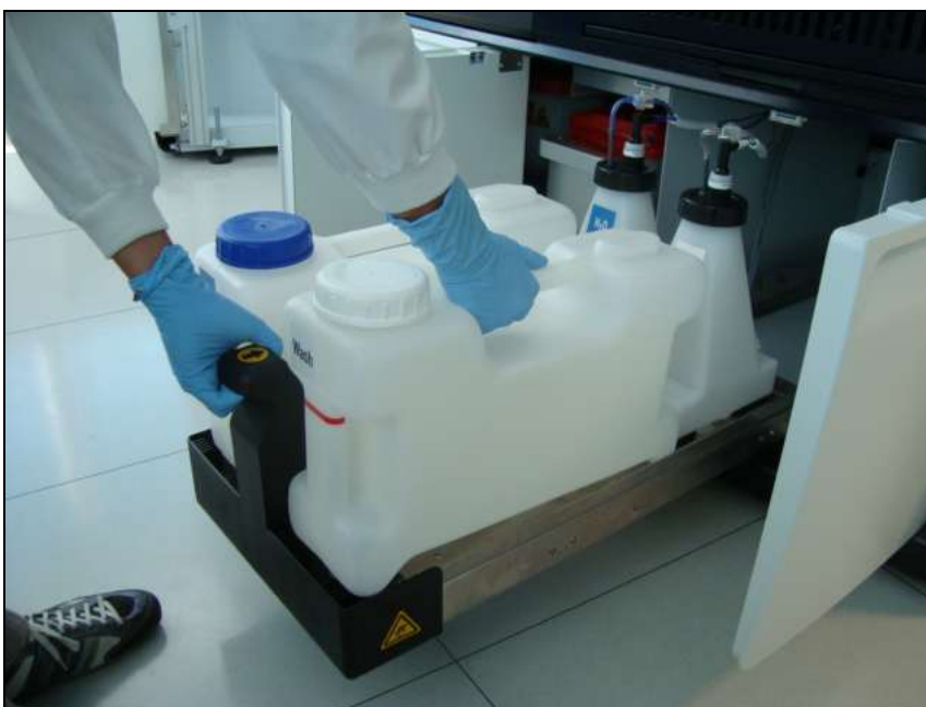
Figure 5-16: Wash buffer tank insertion
