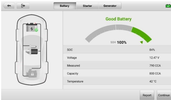
Figure 8-6 Battery Test Results Screen
