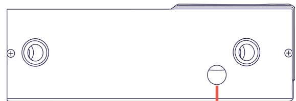
3/4" punchout with Romex connector
