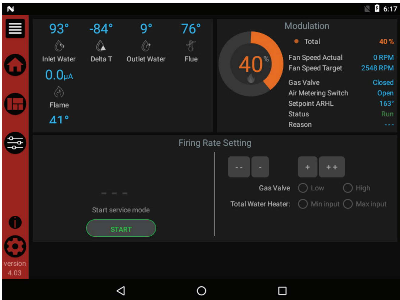
Figure 10-2 Service Maintenance Screen
