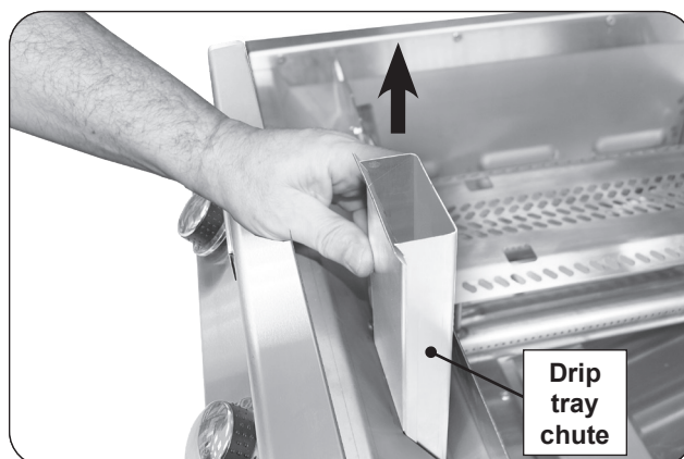
Fig. 41-2 Drip tray chute removal
