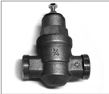
Figure 28 - A Pressure Reducing Valve is required if your home's water pressure is above 80 psi.
