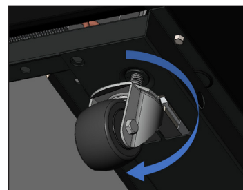
Fig. 8. Position multiple shims at 90° angles.
