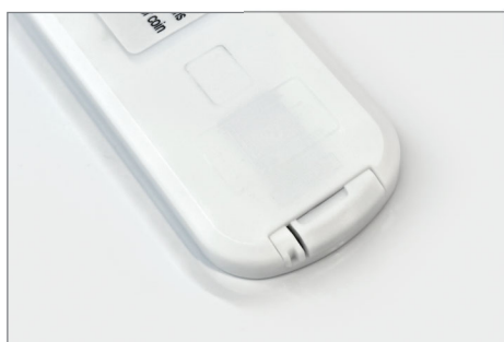
Pull Out the Battery Insulation Tab
