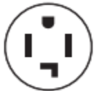
4-wire receptacle (14-30R)
