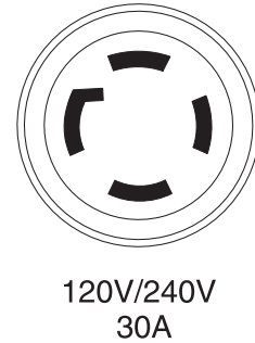
Figure 7 - 120/240 VAC, 30 Amp Receptacle
