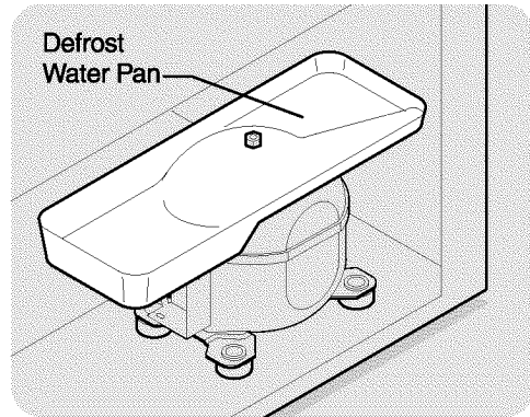
Nonremovable Defrost Water Pan (some models)
