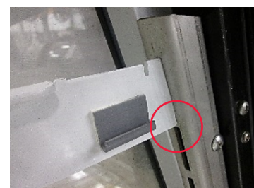
Bottom notch installed (no gap)
