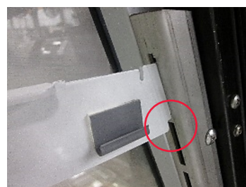
Top notch installed (gap)
