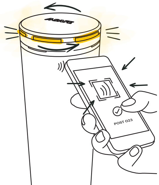
6. The inspector scans the RFID tag of the post to verify location.
