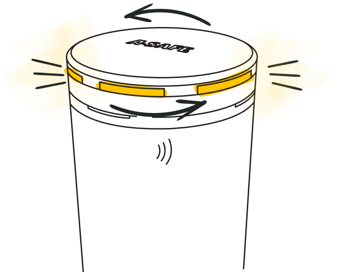
8. Smart Cap opens for DECT registration automatically if not already registered. This is indicated on the Halo.
