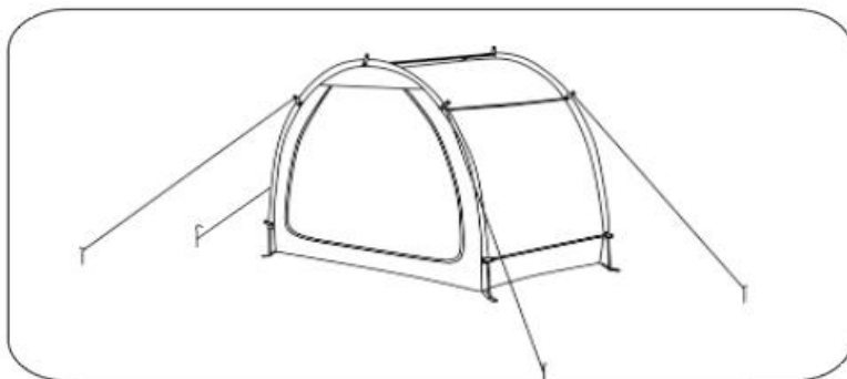
STEP-5: Fixed wind rope ground nail
