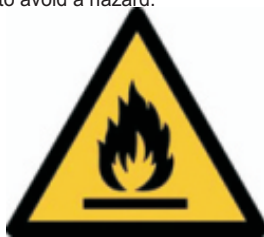
Caution, risk of fire
