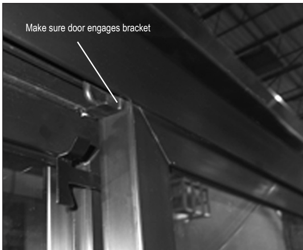
Figure 14: Removing/Installing Sliding Door
