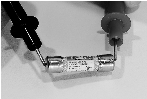
Figure 10. Fuse Test - Ohmmeter Method
