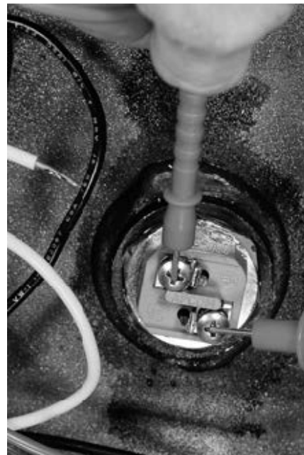
Figure 20. Element Resistance (ohms) Test
