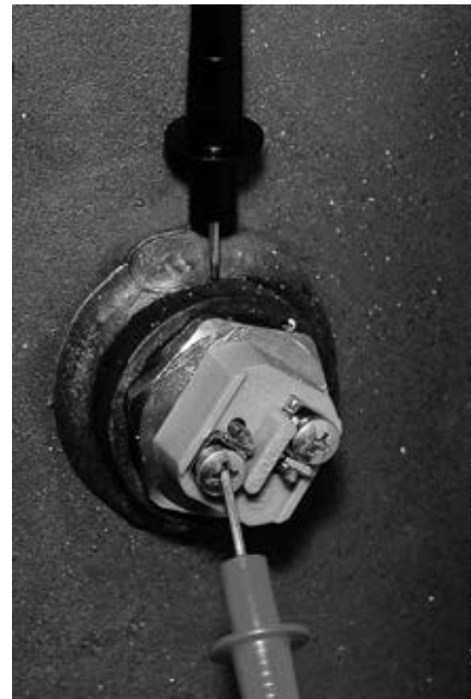
Figure 21. Element Resistance (ohms) Test
