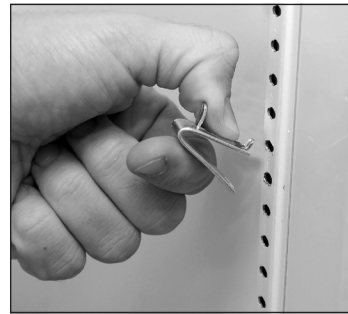
Fig. 1. Installing top tab of shelf clip.
