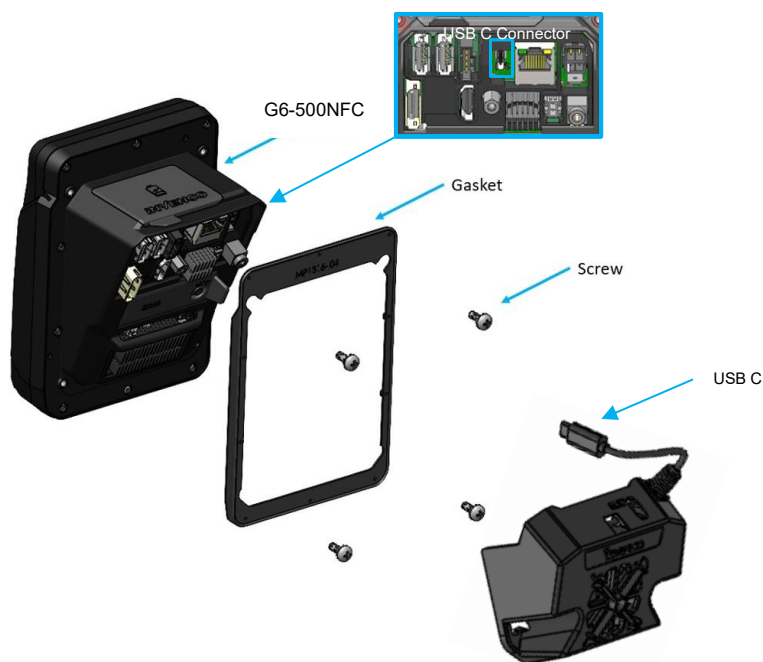
Mounting G6-500NFC onto the dispenser
