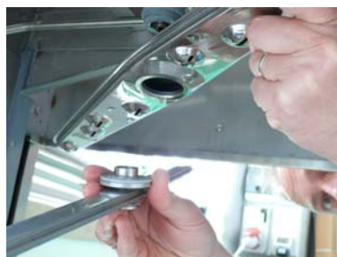
Remove the reel clearing top
