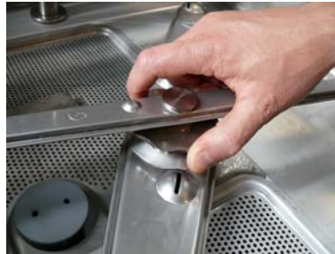
Unscrew the reel rinse lower
