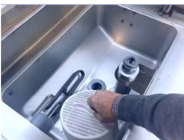
Insert the filter pump suction
