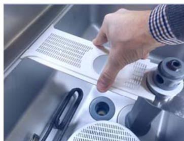
Insert the central support
