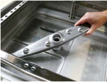
Replace the lower washing arm
