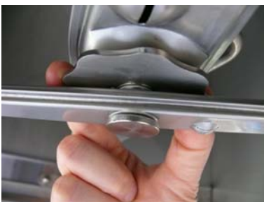
Unscrew the reel rinse top.
