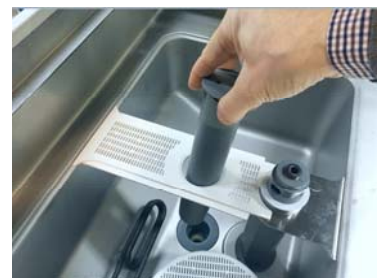
Insert the overflow
