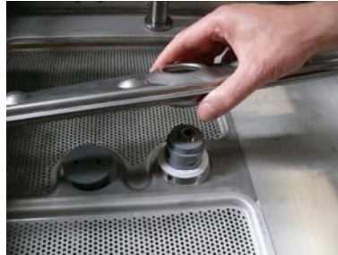
Remove the washing lower reel
