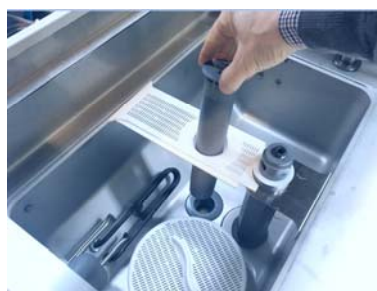
Remove the overflow pipe
