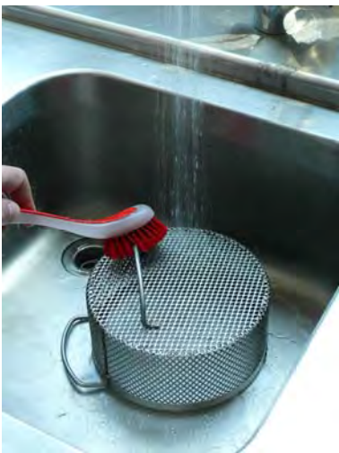
Clean the pump inlet filter by means of a brush
