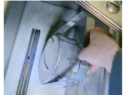
Remove the filter suction pump
