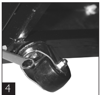
Tighten castor in position with castor wrench.
