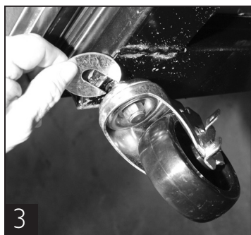
Use shims as necessary to level cabinet.
