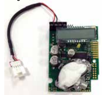
Figure 5: CO2 Sensor PCB.
