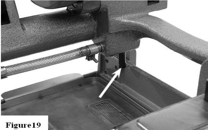
Figure 19. Fluid flow location with threading dies up
