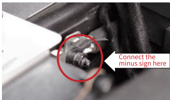
1.4 Connect the negative power terminal.
