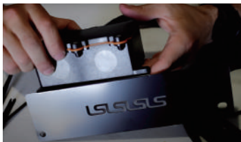
1.1 Attach the power distribution box to the metal bracket(s).
