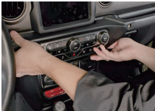
6.2 Put the top panel back on.
