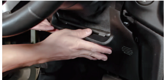
5.6 Put the black plastic panel back on.
