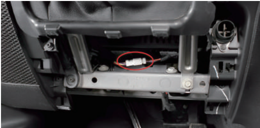
5.4 Run the wire harness behind the dash.
