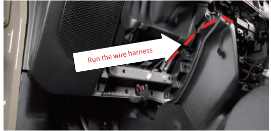
5.5 Connect to the relay harness and ziptie it.
