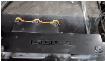
1.3 Mount the bracket(s) with the power distribution.
