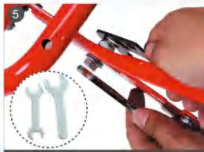
5. Tighten the screws.
