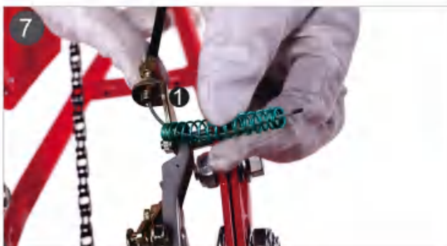
7. Put on the brake spring.
