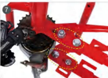
7. All screws and nuts are tightened.
