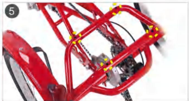
5. Four holes for fixing basket.
