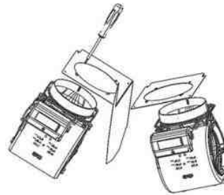
Figure C: Connect Blowers Install dual 600 CFM blowers onto hood with included hardware. Connect molex connectors to blowers.
