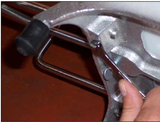
Figure 4. Pusher Head Adjustment Through the Blades.
