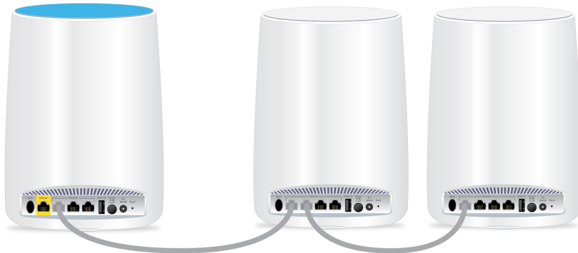
Figure 13. Satellite 1 connected to router and satellite 2 connected to satellite 1
