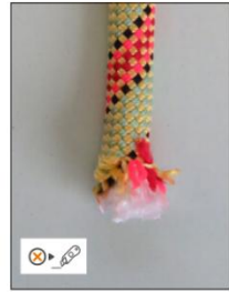
• Damaged rope end
