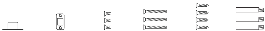
Strike Box x1 Strike Plate x1 M4x8mm x3 M4x30mm x3 M5x20mm x4 Cross bolt x3
