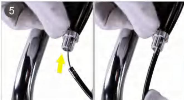
5. Insert the brake tube into the brake lever.
