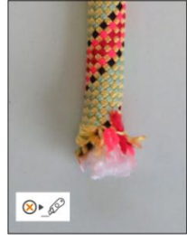
• Damaged rope end
