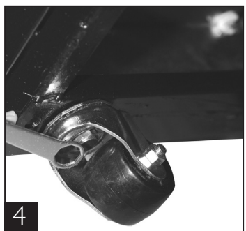
Tighten castor in position with castor wrench.
