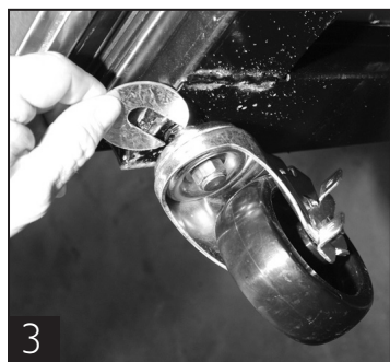
Use shims as necessary to level cabinet.
