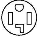
4-wire receptacle (14-30R)
