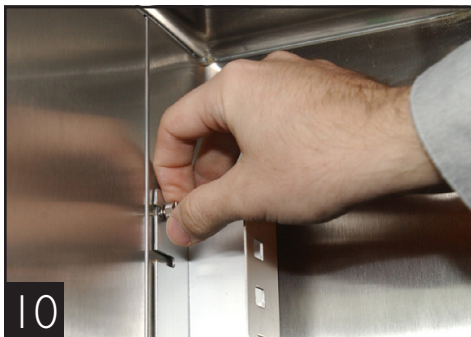
Pilaster installation (side wall of cabinet)
